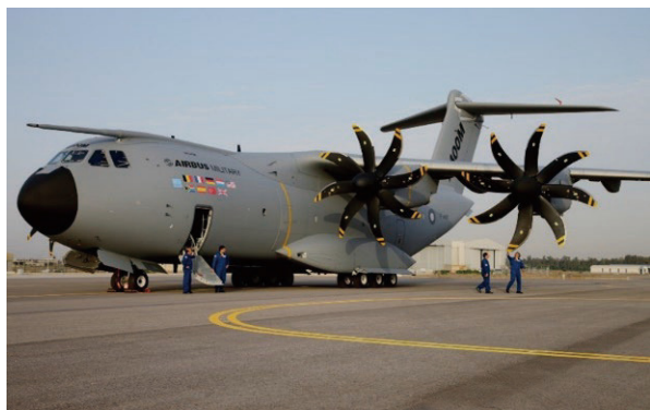
图3 采用4发对转布局的A400M战术运输机 Fig. 3 A400M tactical transport aircraft with 4-engine contra-rotating layout
