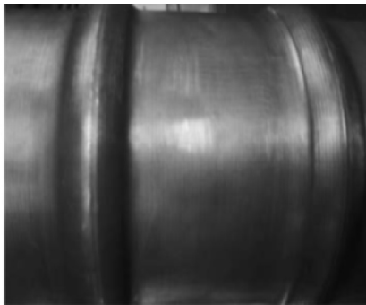
Fig. 14 Formed corrugated tube with optimized processing parameters 20 .
