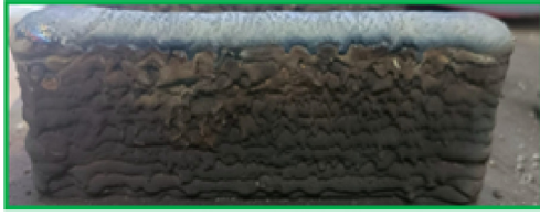
Fig. 4. Wall printed without defects using well-established parameters that have been controlled during the deposition.
