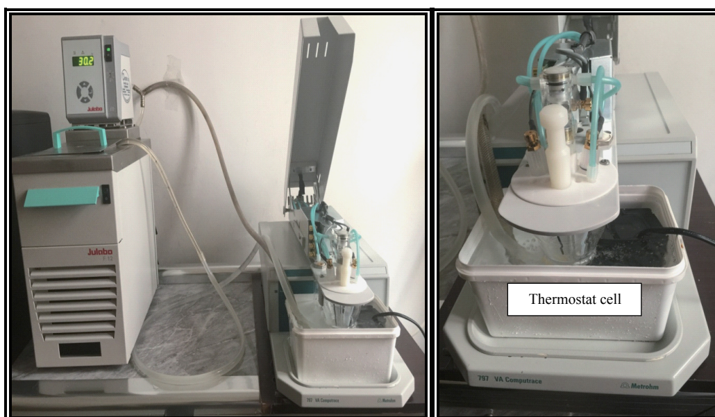
Fig. 1 The modified thermostat cell in polarographic analyzer, 797VA Computrace.
