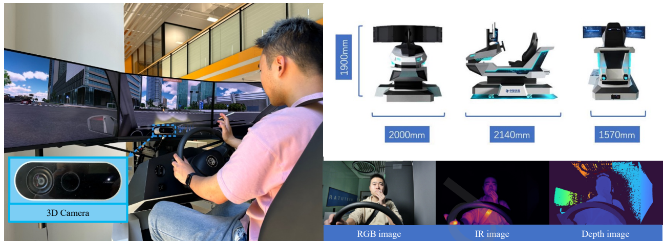
Fig. 4 Intelligent cockpit data acquisition platform equipped with the Orbbec Femto-Bolt camera and representative data samples.
