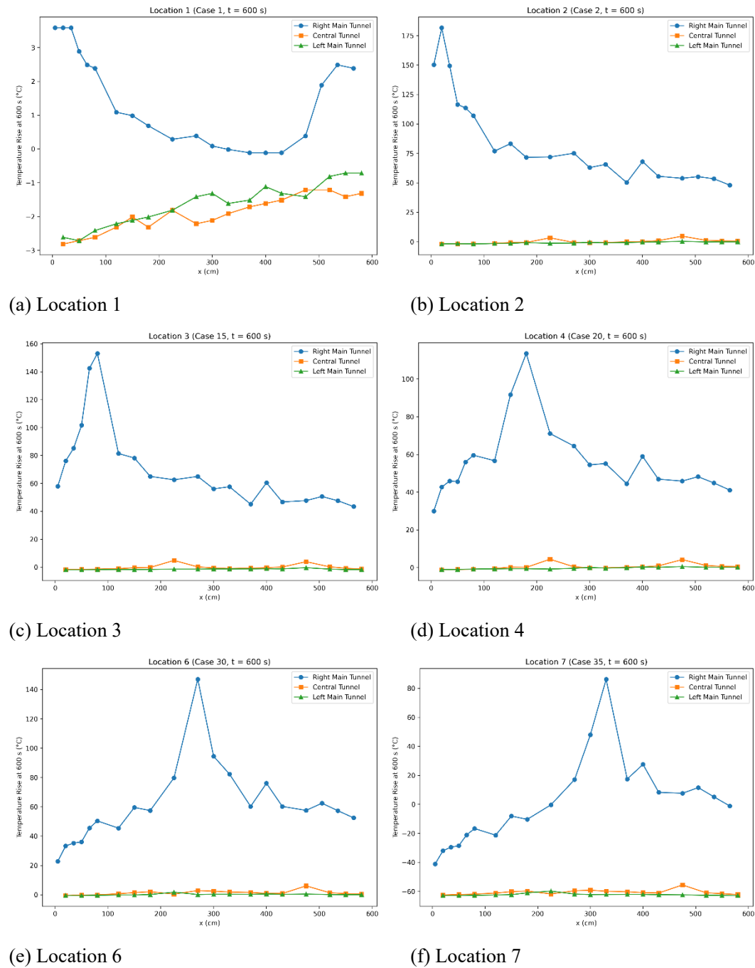
Figure 6 Temperature Comparison of Three Tunnels
