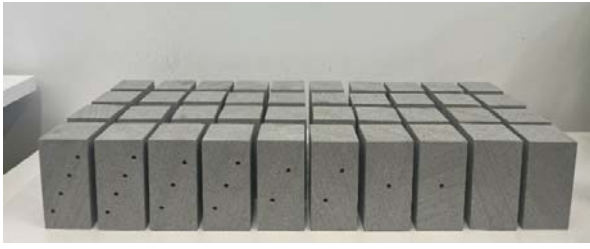
Fig. 2 Standard sandstone samples with cavities
