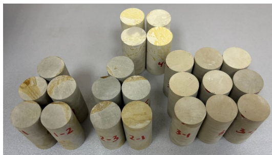
Fig.4 Cylindrical samples of silicites, silicified dolomites and opoka for uniaxial compression
