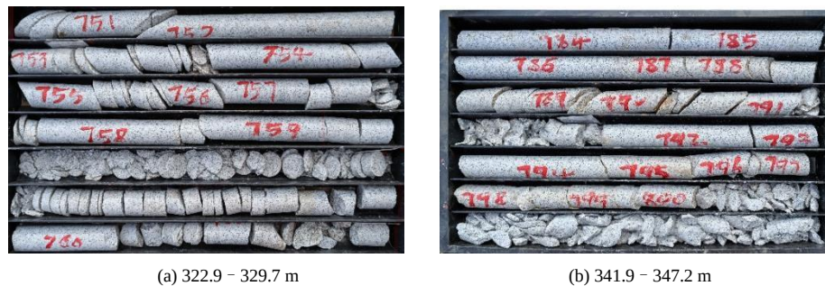
Fig.6 Core discing and crushed zone for borehole ZKJ01
