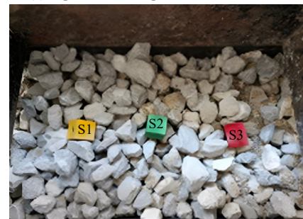
(b) Sensors arranged at equal intervals along the shear direction
