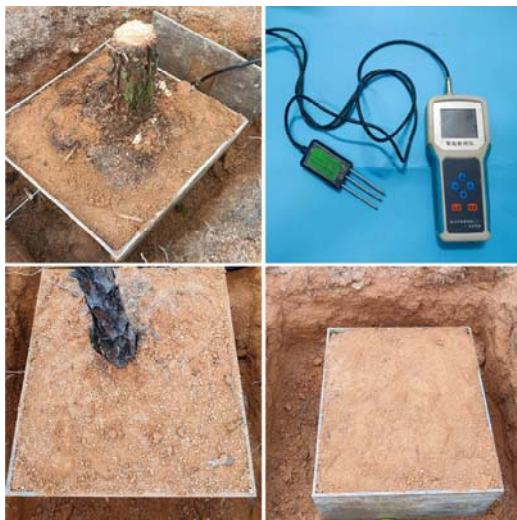
Fig. 4 In-situ shear and moisture content sensor
