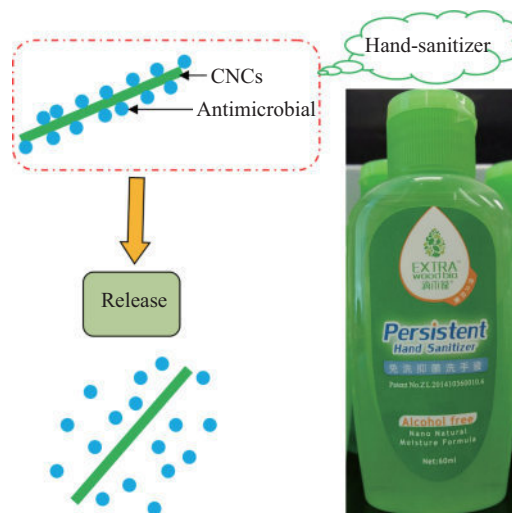
Fig.9 Release behavior of the CNC-based hand sanitizer materials, the development of cellulose-based functional composite products for different applications will move forward, which is partially driven by the demand from consumers for green and healthy living.
