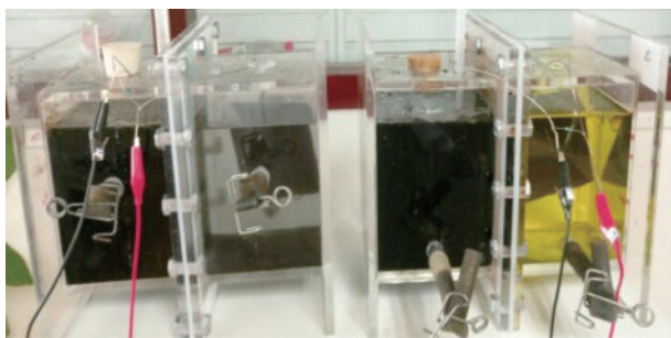
Fig.2 Lab-scale MFC set-up with different cathodic redox solutions
