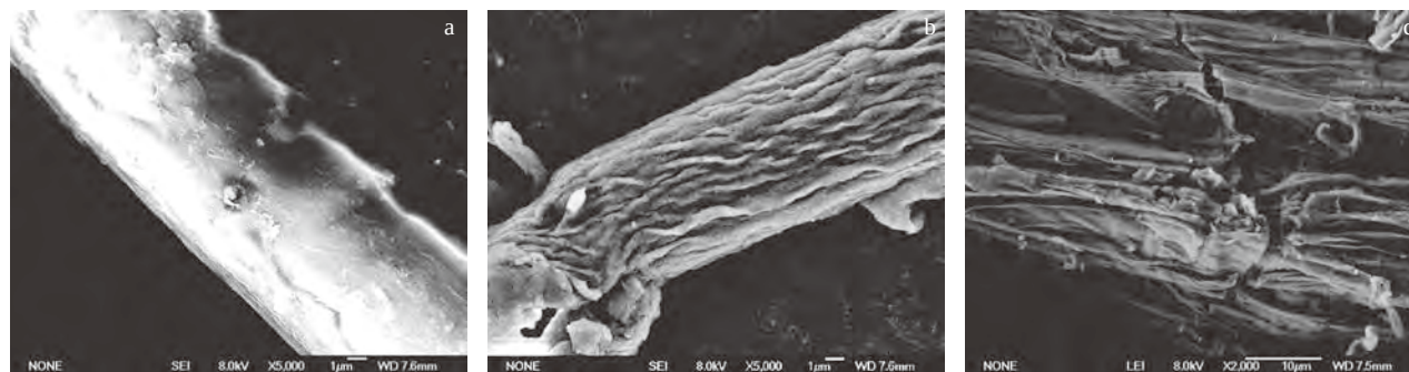
Fig.5 SEM micrographs of the ginger stalk cellulose (a), cellulose extracted by KOH treatment (b), and cellulose extracted by NAE treatment (c)
