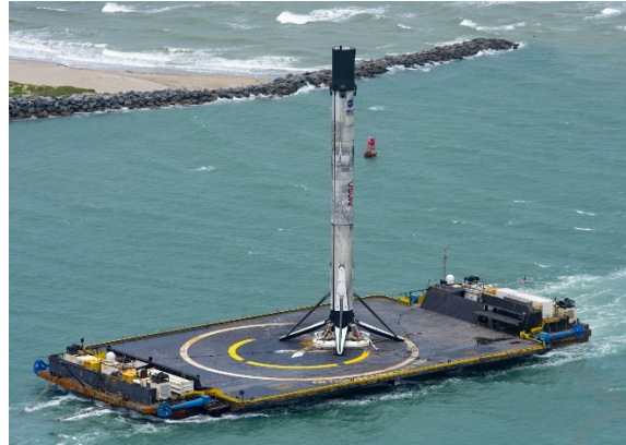
Fig.25 Air-sea recovery of ULV on an autonomous recovery platform [141].
