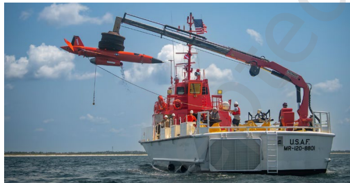
Fig. 24 UAV recovery via robotic retrieval [140].
