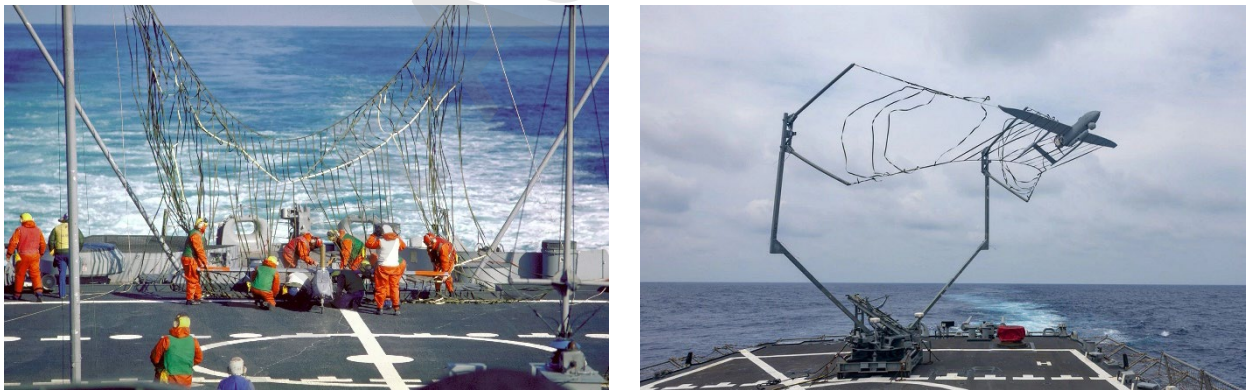
Fig. 23 Shipborne UAV recovery based on flexible net capture [138-139].
