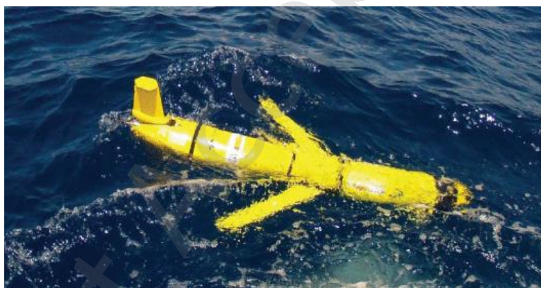
Figure 8 A Slocum G2 operated by PLOCAN (Reproduced with permission from Ref. [182] ©2018, IEEE)
