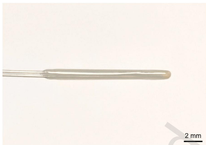
Figure S14. Optical photograph of a fiber Zn//Zn symmetric cell with electro-induced in-situ hybrid hydrogel electrolyte.
