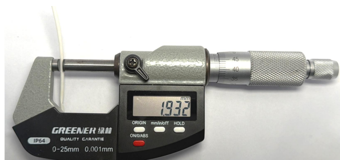
Figure S31. Photograph of a Zn//PANI fiber battery with a diameter of 1.93 mm.
