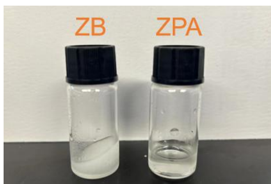
Fig. S21 Electrolytes after resting at -10°C for 24 h.
