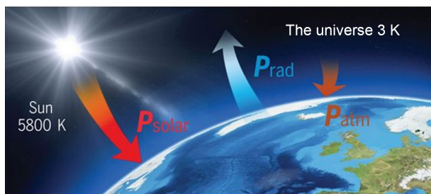
Figure 2 Schematic diagram of the Earth's surface radiative heat flux. Reproduced with permission from Ref. [27], © Yin, X. B. et al. 2020.
