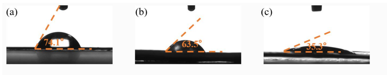
Figure S21 Contact angles of (a) bare Sn, (b) PAM-Sn, and (c) PAM@MXene-Sn electrodes with 3M MSA + 1 M Sn (MSA) 2 .
