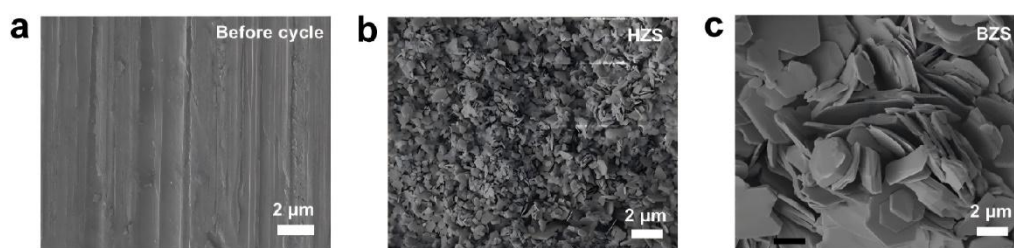
Fig. S9. (a) SEM image of Zn anode before cycling. SEM images of cycled Zn anodes (50 cycles, 10 \text{ mA cm}^{-2}/1 \text{ mAh cm}^{-2} ) in (b) HZS electrolyte and (c) BZS electrolyte.
