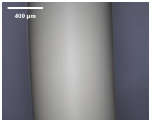
Figure S1. The polarizing microscope image of hydrogel fibers.
