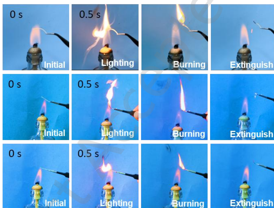
Figure S35. Photographs of ATAFs in flame retardant test, ATAF-H 2 O (top), ATAF-B (middle), and ATAF-BSi (bottom).
