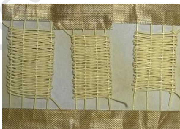
Figure S29. The photograph of ATAF 20 , ATAF 30 and ATAF 40 textiles after the test on a hot plate at 200 °C.
