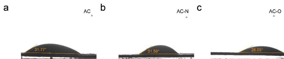
Figure S4. (a-c) Contact angle measurements of AC (a), AC-N (b), and AC-O (c).
