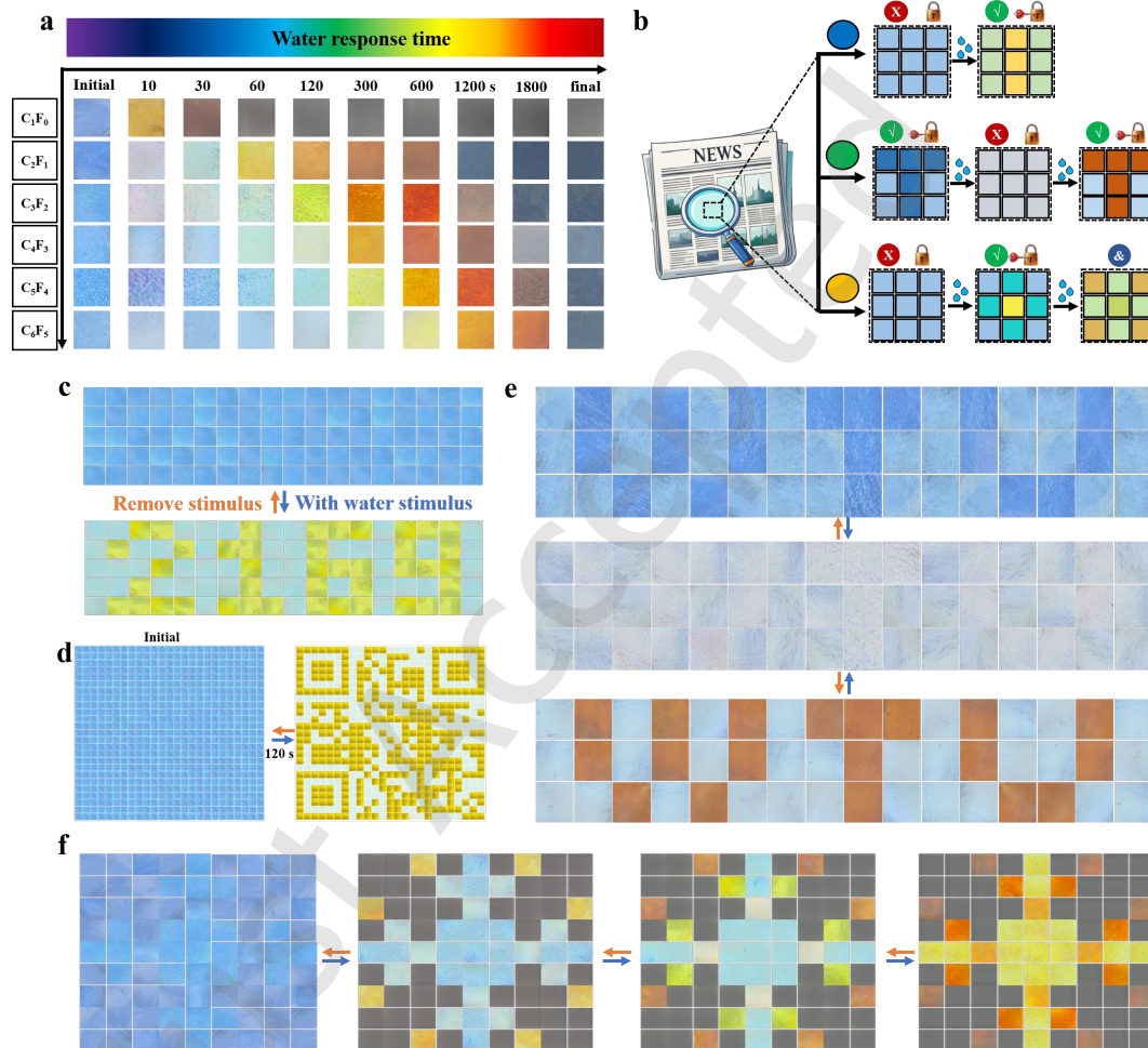
Figure 5 (a) Photos of the color-changing response with water stimulated for different laminate blocks. (b) Three models of information encryption and decryption based on photonic matrix. (c, d) Photonic matrix comprised by C3F2 and C5F4 blocks for model I-type information encryption and decryption. (e) Photonic matrix comprised by C2F1 and C6F5 blocks for model II-type information encryption and decryption. (f) Photonic matrix comprised by C1F0, C2F1, C3F2, C4F3, and C5F4 blocks for model III-type information encryption and decryption.
