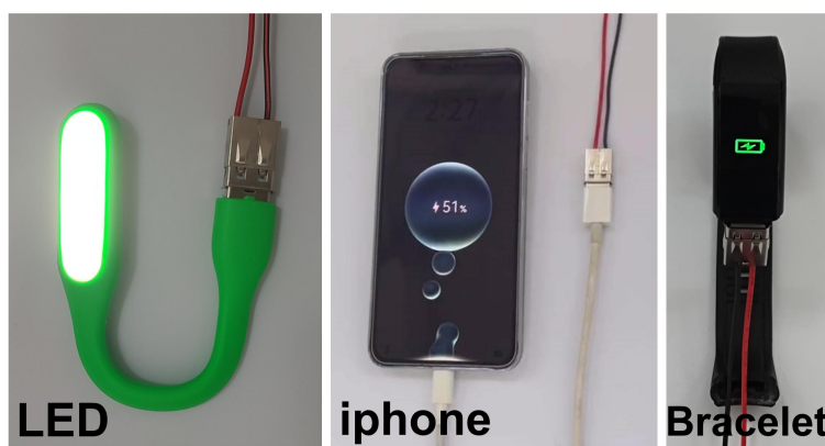
Figure S12 The PMG 1 -loaded STEG can energize various electronic equipment, including the LED, mobile phone, and smart bracelet with the passive voltage booster.
