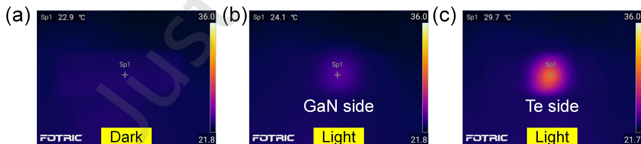
Figure S14 (a) Thermal images of the device surface in the dark state, (b) under 365 nm illumination on the GaN area, and (c) on the Te area.
