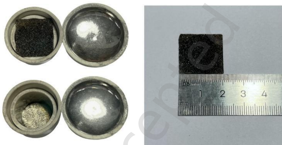
Figure S14 Digital photographs of the crucible used for Pt/NiO/NF(Ga) synthesis (30 mg \text{Pt}(\text{acac})_2 , 1 mL Ga, deposition height: 2 cm).
