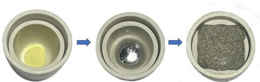
Figure S13 Digital photographs illustrating the synthesis process of Pt/NiO/NF(Ga).
