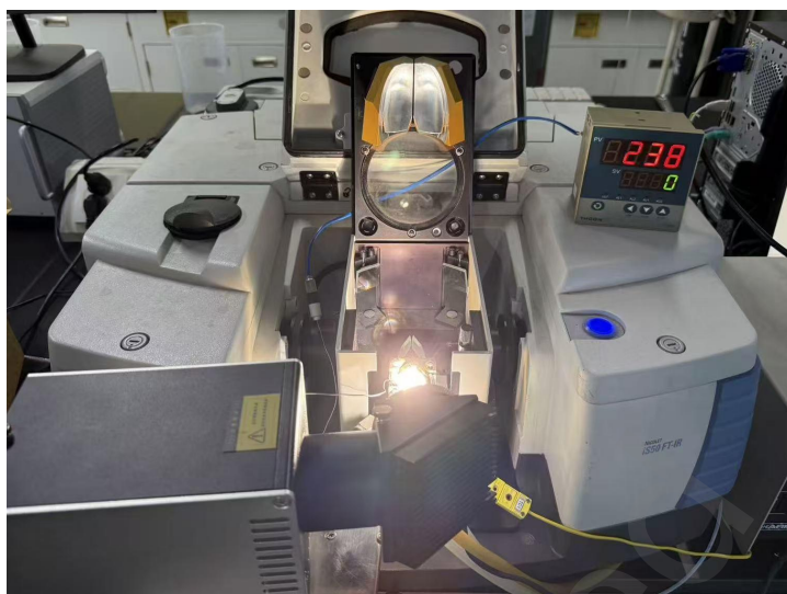
Figure S16. Photograph of the in-situ DRIFTS reactor during light driven process, showing the measured temperature of catalyst surface (via thermocouple) under illumination.
