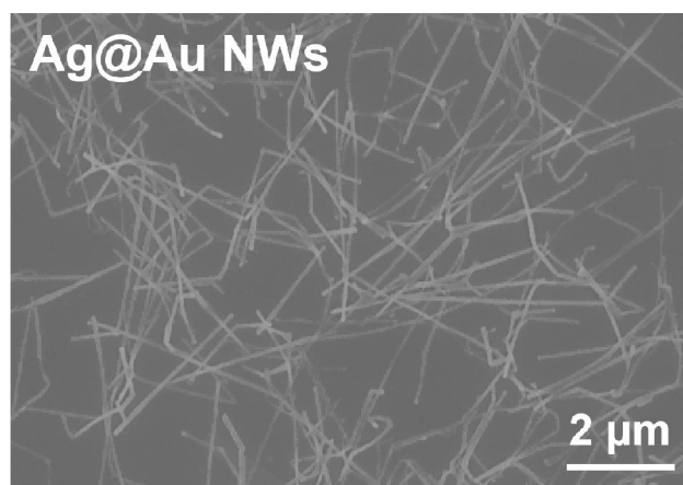
Figure S19. SEM images of AgNWs (left) and Ag@Au NWs (right) after \text{H}_2\text{O}_2 treatment.
