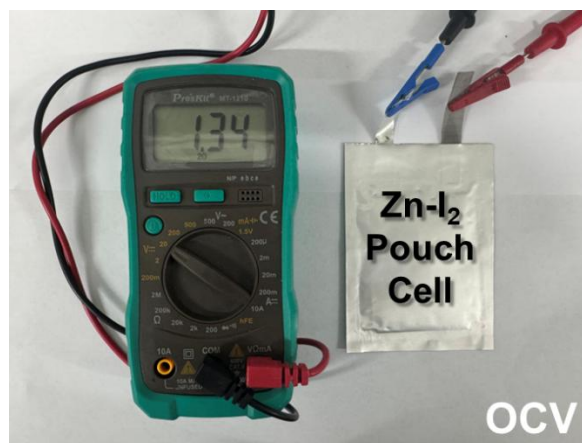
Figure S24. Open circuit voltage (OCV) of Zn-I 2 pouch cell.
