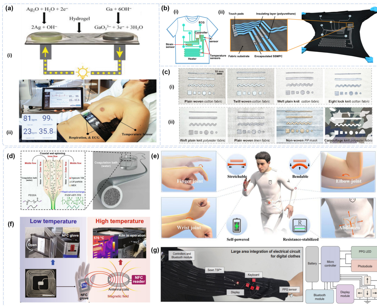
Figure 12 Application of printed batteries and E-textiles. (a) Printed battery: (i) schematic diagram of structure and working mechanism; (ii) biomonitoring wearable belt powered by multiple stretchable batteries for acquiring body temperature, respiration and heart monitoring. Reproduced with permission from Ref. [38], © Wiley-VCH GmbH 2022. (b) Integrated wearable T-shirt: (i) a schematic shows the highly integrated T-shirt; (ii) photograph of the printed T-shirt for smart wearables. Reproduced with permission from Ref. [49], © American Chemical Society 2019. (c) Universal printability of the LMPs-Ag-SISI-EVA composite to adapt to textiles with (i) different structures and (ii) various materials. Reproduced with permission from Ref. [157], © American Chemical Society 2024. (d) Wet spinning for fabricating continuous fiber. Reproduced with permission from Ref. [143], © Zheng, L. J. et al. 2021. (e) Novel passive E-textile for mechanical motion sensing. Reproduced with permission from Ref. [196], © Wiley-VCH GmbH 2025. (f) E-textile for outdoor access control operation in winter and door access of a kiln in operation under extreme temperature. Reproduced with permission from Ref. [161], © Zhang, Y. et al. 2025. (g) Photograph (left) and circuit schematic (right) of E-textile based on twisted fibers. Reproduced with permission from Ref. [190], © Lee, G. H. et al. 2025.
