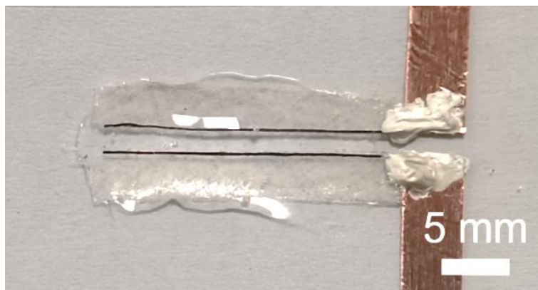
Figure S13. The digital image of an assembled MF-based supercapacitor.
