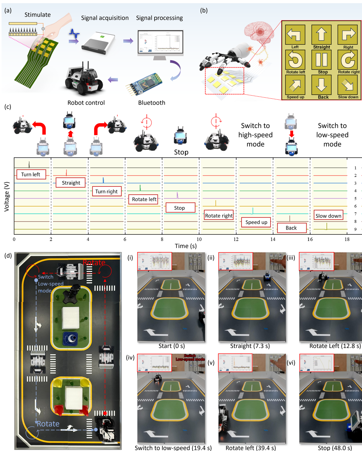
Figure 5 Application of MN-TPS based wearable interactive platform for robot control. (a) Working principle of MN-TPS based wearable interactive platform for robot manipulation. A pressing signal can be converted into a trigger signal to control the appliances. (b) Schematic diagram of the interactive platform with nine control buttons for specific functions. (c) Output signal waveforms from each of the nine specific-function buttons. (d) Screenshot of the wirelessly controlled smart mobile robot performing the programmed task.
