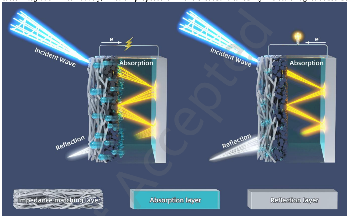
Figure 1. Schematic illustration of the mechanism of electrochemically-driving tunable microwave absorption device.
