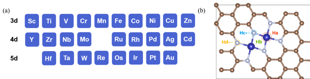
Figure 1 (a) Metal elements considered to construct M 2 -N 6 -graphene slab model in this work. (b) Top view of the M 2 -N 6 -graphene slab model as well as the adsorption sites for hydrogen.
