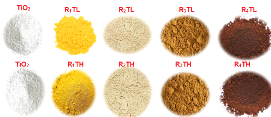
Fig. 2 Images of TiO 2 NPs, 0.1-wt% Ru/TiO 2 (R 1 TH), 0.2-wt% Ru/TiO 2 (R 2 TH), 0.3-wt% Ru/TiO 2 (R 3 TH), and 0.4-wt% Ru/TiO 2 (R 4 TH) synthesized via hydrothermal method (First line). TiO 2 NPs, 0.1-wt% Ru/TiO 2 (R 1 TL), 0.2-wt% Ru/TiO 2 (R 2 TL), 0.3-wt% Ru/TiO 2 (R 3 TL), and 0.4-wt% Ru/TiO 2 (R 4 TL) synthesized via IL-assisted hydrothermal method (Second line).
