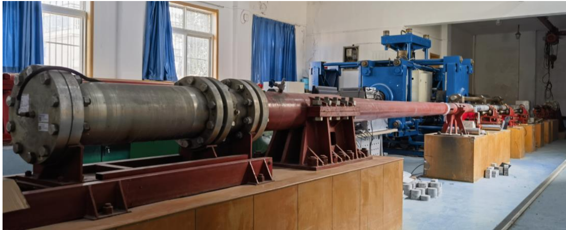
Fig. 2. \Phi 100 mm SHPB test equipment.
