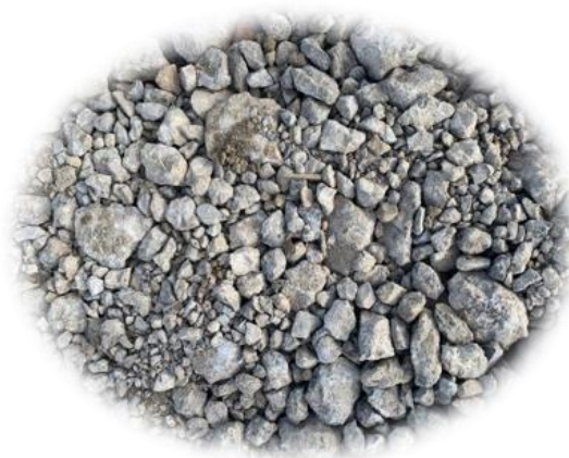
Fig. 9. Apparent morphology of construction waste.
