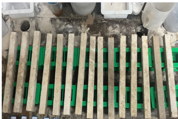
Fig. 2. The specimens of flowable solidified soil after drying shrinkage curing.
