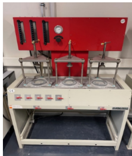
Fig. 2. Water permeability device.
