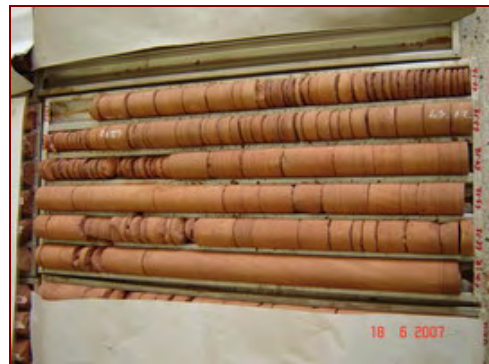
Fig.6 Fracture Zone in Massive Sandstone, Interbedded with Thin Shale
