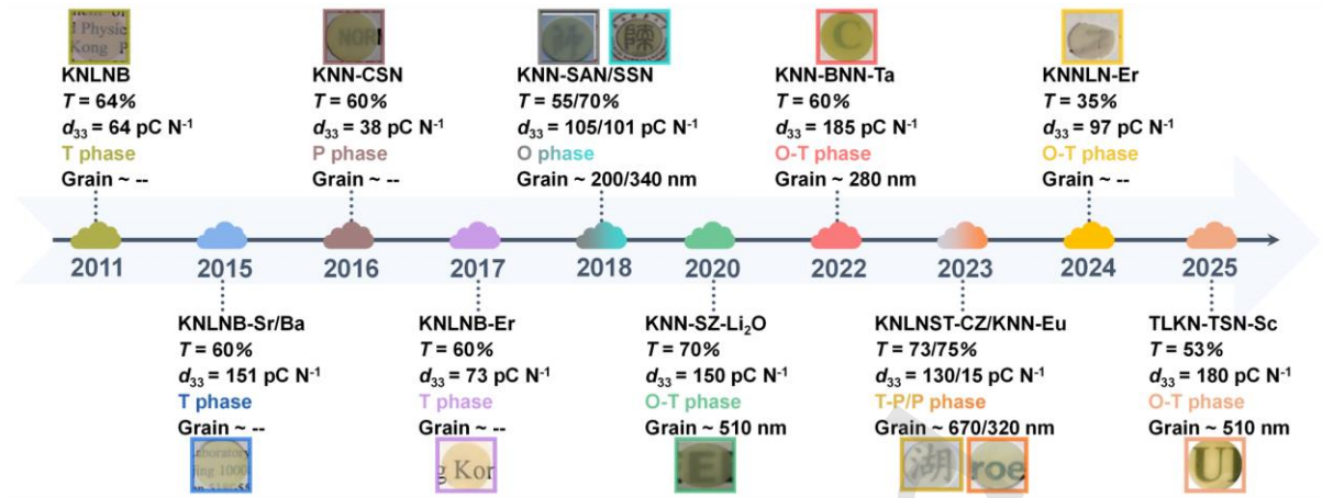
Fig. 12. Research progress on KNN-based transparent piezoelectric ceramics.
