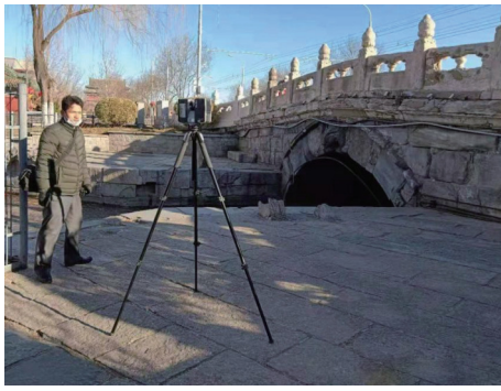
Fig. 11 On-site laser scanning operation.
