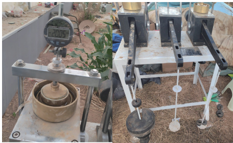
Fig. 2 Field consolidation test of foundational soil.
