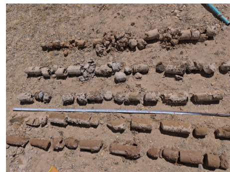
Fig. 1 Distribution of soil samples from field boreholes.
