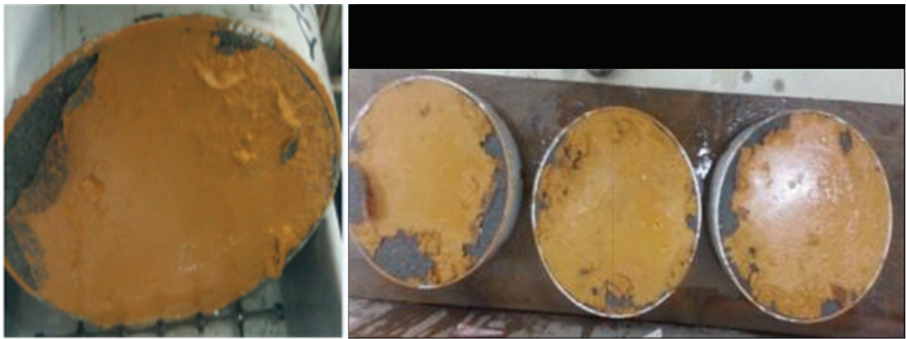
Fig. 4 Coating A after 25 freeze-thaw cycles
