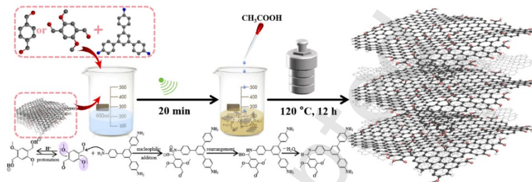
Figure 1 Schematic diagram of the fabrication process of TADM/GO and TATP/GO.
