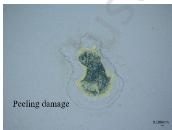
Fig.10 Micrograph of the F 3 coating after impact at 776 m/s
