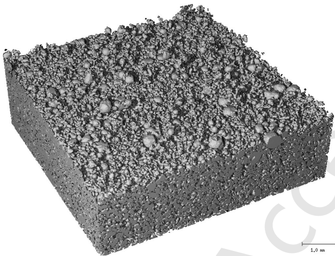
Figure 3. Micro-CT image of snow surface at a temperature of -19.1\text{ }^{\circ}\text{C} after the 20 runs [25].
