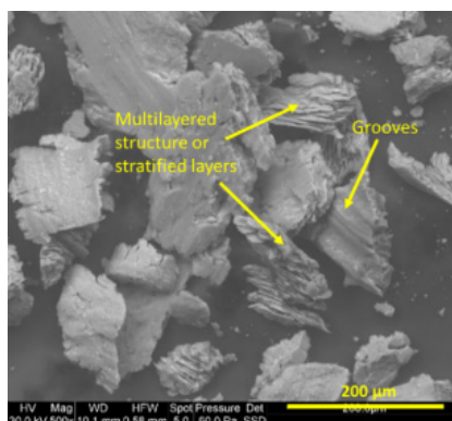
Fig. 12 Morphology of debris caused between 5 and 10 m (50–100 s).
