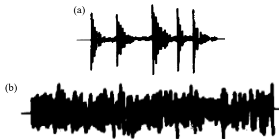
Fig. 7 Waveform of AE signals: (a) burst AE signal; (b) continuous AE signal.
